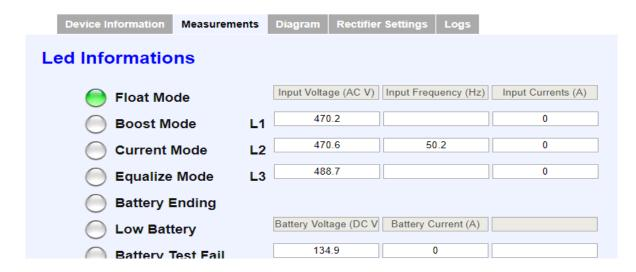
Remote monitoring and control of devices such as UPS, Rectifier, Stabilizer via web server can be done through web browser without any interface. The TCP network is used in these controls and only the IP address of the device to be connected is known and can connect to any number of client web servers and control and monitor the process easily.
