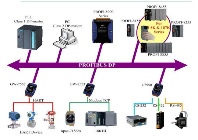
PROFIBUS (Process Field Bus) is a standard for fieldbus communication in automation technology and was first promoted in 1989 by BMBF (German department of education and research) and then used by Siemens. It should not be confused with the PROFINET standard for Industrial Ethernet. PROFIBUS is openly published as part of IEC 61158.
