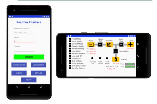
Thanks to the android application, it is now very easy to remotely monitor and control ups, rectifiers. In addition to the Modbus tcp protocol, the service can be used in different protocols. You can install apk file on any phone with Android operating system and do everything functional like battery status, voltage information and power on and off of your UPS.you can even monitor the device from outside the city if you want.
