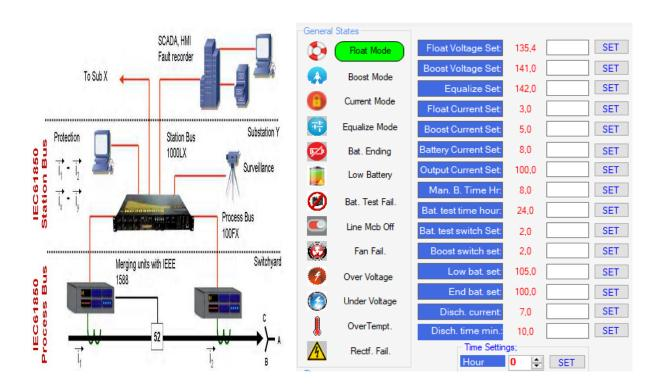
IEC 61850 is an international standard defining communication protocols for intelligent electronic devices at electrical substations. It is a part of the International Electrotechnical Commission's Technical Committee 57 reference architecture for electric power systems. it can be used safely in power electronics devices in line with the developing needs.
